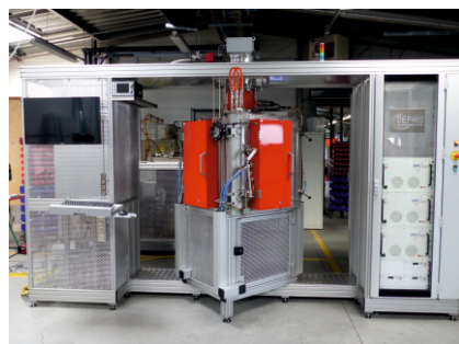
P9/P10: DEPHIS' latest hybrid coating reactor the TriProS, which combines the HiPIMS, Arc, CVD, DC-P technologies into a single cost effective machine. The machine is equipped with SPIK3000A generators in a bipolar configuration.
